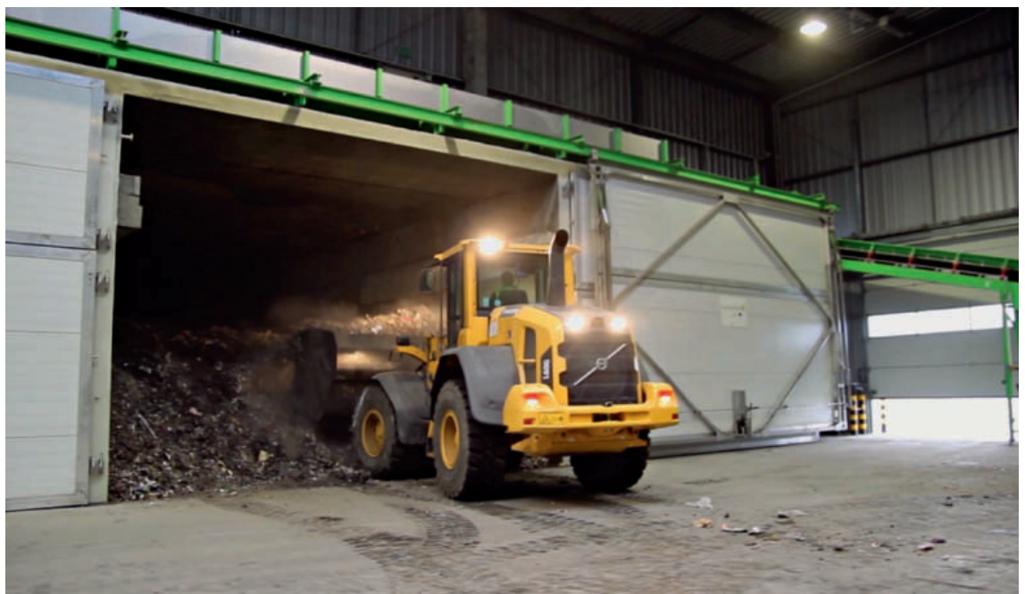
Emptying of the rotting tunnels ▶
